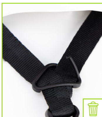
Broken lateral divider
