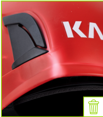
Deformed external shell
