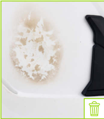
External shell with traces of chemical substance
