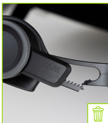
Broken adjustment system branch
