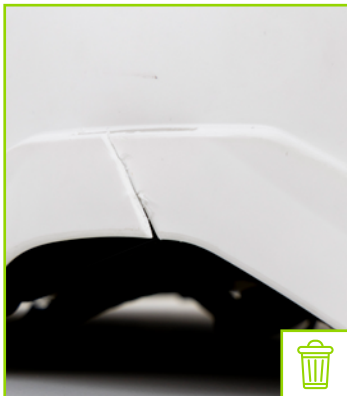
Cracked accessory slot
