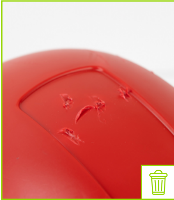
External shell with impact deformation
