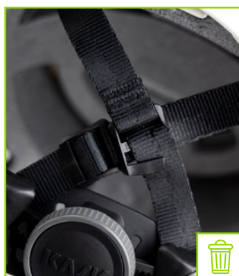
Broken rear adjustment buckle
