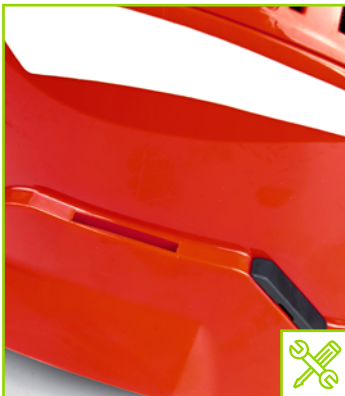
Accessory slot missing cap
