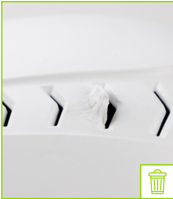
Shell with deformed ventilation hole
