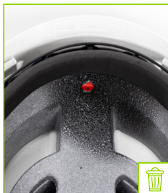
Inner shell with flame burn marks
