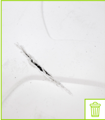
Cracked external shell
