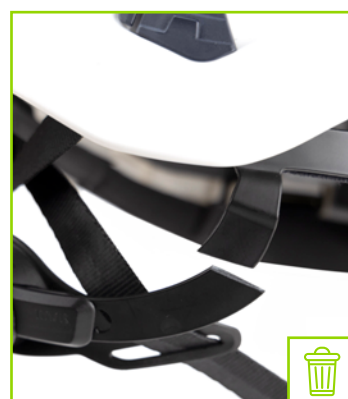
Broken regulation system branch
