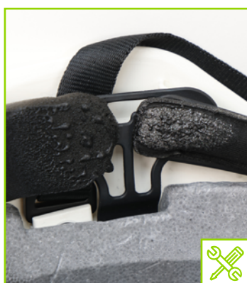
Liner with flame burn marks
